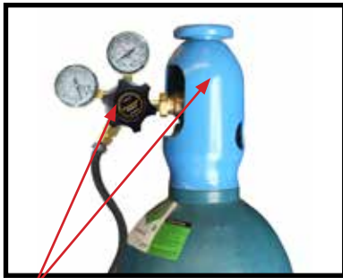
(7) Carefully open the valve of the gas cylinder, set the flow to 6-10 l/min
