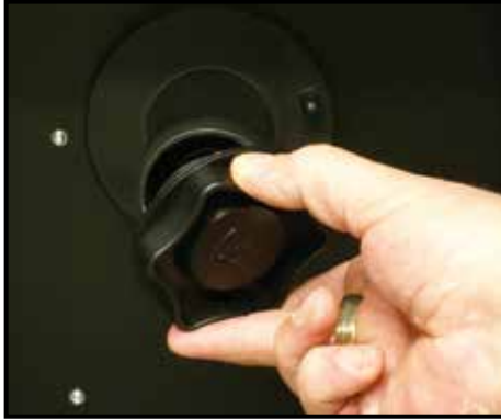
(1) Remove the spool retaining nut.
