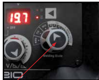
(17) Smartset is a predefined setting based on Gas and wire used. The machine will preselect Voltage and wire speed allowing the user to quickly find the best welding parameters for a given metal.
