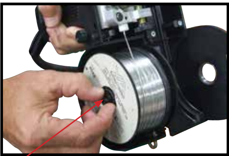
(12) Adjust spool holder tension
