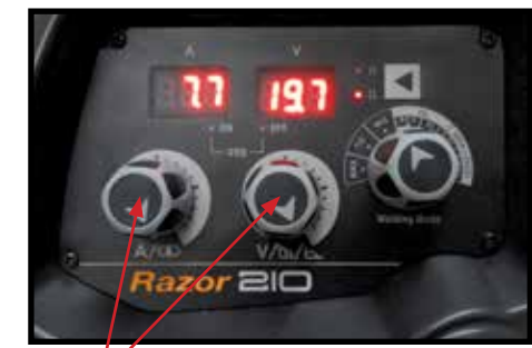
(17) Set welding parameters using the voltage and wire feed controls.
