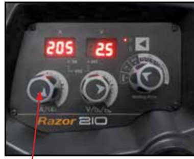
(8) Set the welding current using the amperage control dial
