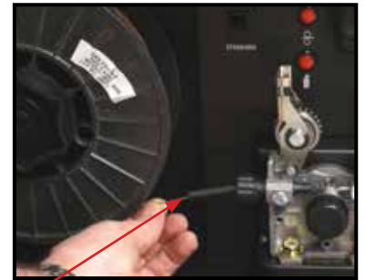
(7) Place aluminum wire onto spool holder. Feed the wire through the inlet guide tube on to the drive roller. NOTE: MIG 180-145 not geared
