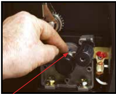
(8) Feed wire over the drive roller into the outlet guide tube, Push the wire through approx 8-9in. Use a Knurled Drive Roller of the correct size
