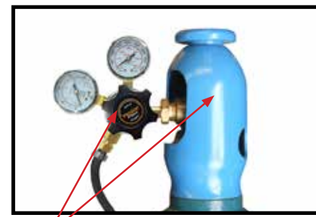
(16) Carefully open the valve of the gas cylinder, set the flow to 12-15 l/min
